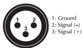
DMX-input XLR mounting-plug:
