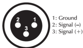
DMX-output XLR mounting-socket:
