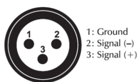
DMX-input XLR mounting-plug:
